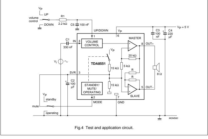
Reduction of the value of capacitor C2 results in a decrease of the SVRR performance at low frequencies (see Fig.9).
